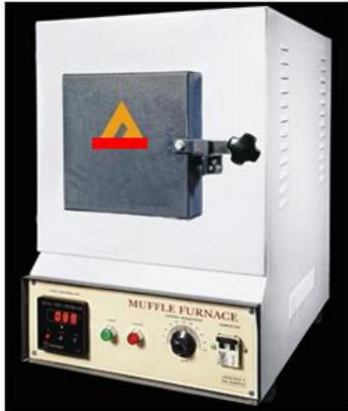
**Construction** : Outer shell of the Muffle Furnace is made of MS sheet fitted on angle iron frame . There is all round insulation by ceramic fiber sheets and blankets for minimum heat loss and low thermal inertia due to light weight of the insulation materials . The door is also thoroughly insulated to obviate any chance of heat leakage through the door .
